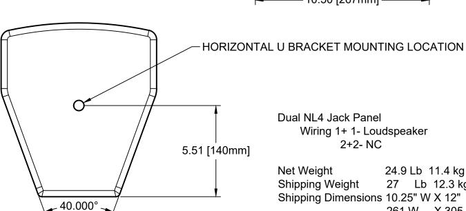
Dual NL4 Jack Panel Wiring 1+ 1- Loudspeaker 2+2- NC
